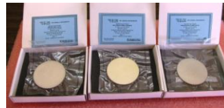
ZnO + 2% Ag Target (99.99%) ZnO Target (99.99%) ZnO + 2% Al Target (99.99%) 3" dia x 3mm thick Bonded to Cu Backing Plates
