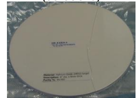
Hafnium Oxide (HfO 2 ) 8" dia x 6mm Target (99.995%)
