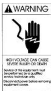
This label indicates a presence of high voltage in or around the equipment, which may cause severe injury or death. All appropriate precautions should be observed when installing, operating or servicing this equipment.
